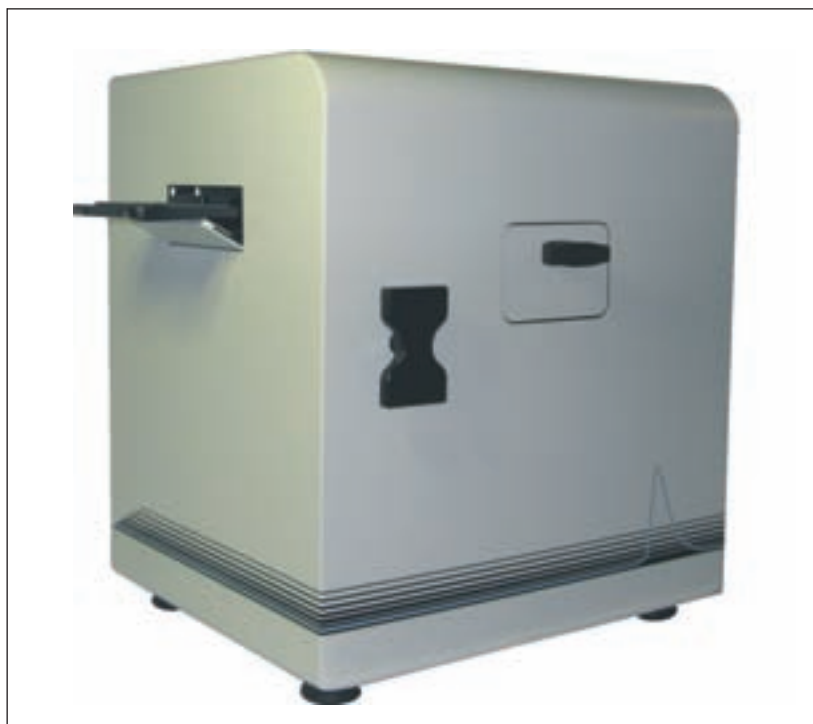
Figure 11: Current version of the two-channel FI2 plate reader equipped with a microchip laser excitation source. Filters are used to isolate either the 532nm or 355nm laser wavelengths for excitation. Each channel has a six-position filter wheel for fluorescence wavelength selection
